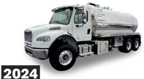
2024 FREIGHTLINER M2 2024 INTERNATIONAL MV607 2500-Gallon Aluminum Vacuum Tank, NVE 607 Vacuum Pump, Cummins L9 300HP Engine, 33,000 GVWR
