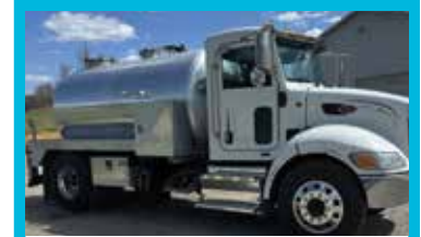
2013 Pete, PX6 Paccar, 294k, Allison Auto, AC, cruise, 26,000 gvw, 2000 gal aluminum tank, 1500/500, Masport HXL75 vac pump, Heavy Duty water pump, 2 pot rack, good tires and aluminum wheels. Very good running truck. Can be opened up for septic. $45,000.00 Hull's Truck Bodies LLC 740-820-5338 (P05)
