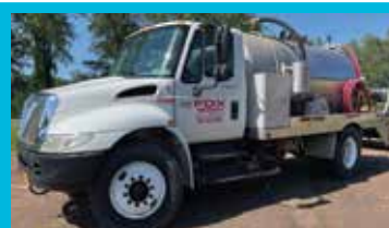
2007 International 4300, DT466, automatic, newly rebuilt Masport HXL75, newly rebuilt hydraulic pump, Best Enterprise stainless tank 1900/400, two unit rack on rear, service toilets from both sides of the truck, good tires, perfect unit to service restroom trailers and holding tanks. We sold our business and the new owner did not need this truck. $39,750. John 601-946-0615 or johnfoxups@gmail.com. Located in MS. (P09)
