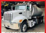
2013 Peterbilt 382 Made to Order. 3,600-gallon steel tank W/Masport Cobra (532 CFM) Cummins ISL 9, 380hp, FR013210C (10-speed Eaton Fuller) 52k GVWR, low air leaf suspension, 201,015 miles. Newly ordered to build. Call: 501-388-0052, email: Ironvac. zach@septictrucks.com. AR (P02)
