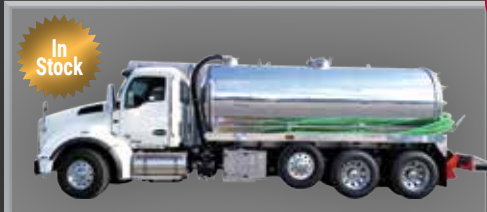
2024 T880 KENWORTH 485HP, ULTRA SHIFT 20/20/46, NVE 4310 BLOWER PACKAGE, 4500 GALLON TANK
