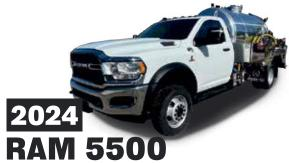
1300-Gallon Aluminum Vacuum Tank, 900 Waste/400 Water, Masport HXL4V Vacuum Pump (160 CFM), 6.7L Cummins Turbo Diesel Engine, 2-Unit Hauler
