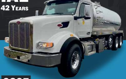
5000-Gallon Aluminum Vacuum Tank, NVE 4310 Blower, **Cummins X-15 500HP Engine**
