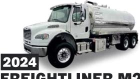
4000-Gallon Aluminum Vacuum Tank, NVE 4310 Blower, Cummins L9 350HP Engine
