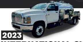
1500-Gallon Aluminum Vacuum Tank, 1000 Waste/500 Water, NVE 304 Vacuum Pump (210 CFM), International 6.6L 350HP Engine
